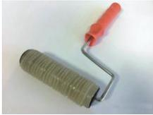
**GRANITE EFFECT:** Dilute with water at 10%-15% (max 5%-10% in cold season). Apply 1 coat of Plasma 3D FUSION uniformly by brush. Smooth it out by stainless trowel to obtain the desired thickness. Work it immediately with a proper roller in a vertical or horizontal way. Once almost dry shave it with a stainless spatula and shine it with cloth or polisher. For major protection and water resistance after 12-48 hours apply 1 or 2 coats of CLEAR<sup>1</sup>.
