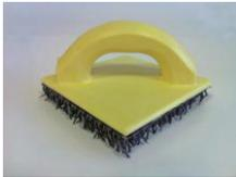
**MARBLE EFFECT:** Dilute with water at 5% (the product is ready to use in the cold season.) Apply 1 uniform coat of Plasma 3D FUSION by brush and work it immediately after by apposite buffer choosing between vertical or horizontal direction. Level it immediately by stainless trowel. Once almost dried polish it with stainless trowel obtaining Marble 3D effect and shine it by cloth or flex machine. For major protection and water resistance apply, after 12-48 hours, 1-2 coats of CLEAR<sup>1</sup>.
