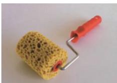
**VIPER EFFECT:** Dilute with water at 5-10% (max 5% in cold season). Apply 1 coat of Plasma 3D FUSION uniformly by brush. Smooth it out by stainless trowel to obtain the desired thickness. Work it immediately with a proper roller in a vertical or horizontal way. Once almost dry shave it with a stainless spatula and shine it with cloth or polisher. For major protection and water resistance after 12-48 hours apply 1 or 2 coats of CLEAR<sup>1</sup>.
